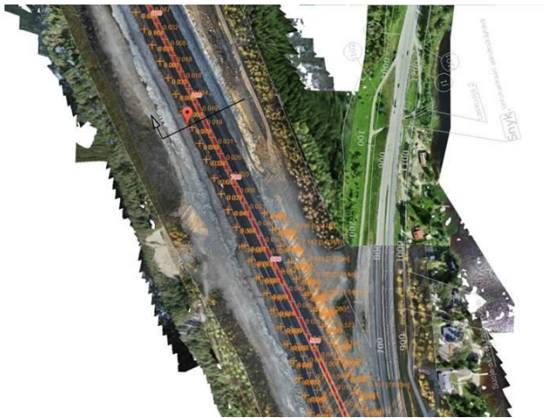
Figure 13. Highway Design and Construction project Vt4 Kirri-Tikkakoski – a BIM model View in Infrakit Cloud Service (Destia Oy).
