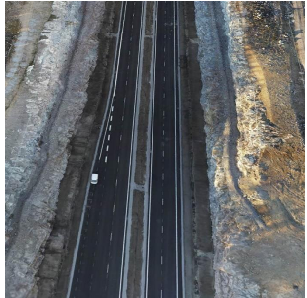
Figure 15. Example – a drone image used for model-based quality control (Destia Oy).
